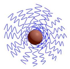
Schematic presentation of the new magnetic vectors: PDMAEMA arms attached to a crystalline iron oxide core stretch in all directions. The nanoparticle thus assumes a star-shaped appearance.
