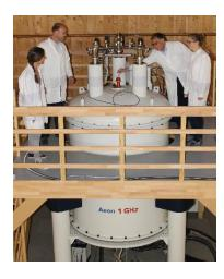
Rösch (second from the right) and members of his team insert a protein sample into the magnet of the 1 GHz spectrometer in order to study the protein's conformation.
