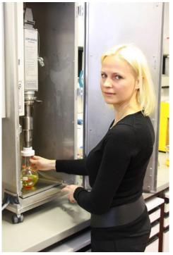
Dr Daria Andreeva demonstrates the procedure of sonication of solid particles in an aqueous suspension by using the UIP1000hd (Hielscher, Germany) horn ultrasound device operated at 20 kHz with a maximal output power of 1000 W.
